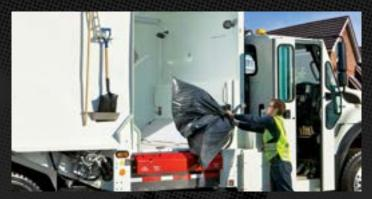
The Expert drop frame configuration is perfect for manual or semi-automated waste or recycling collection, and the loading height of only 5.5" above the chassis frame makes this configuration safer, faster, and easier to load. With the shortest wheelbase in the industry, this truck can easily maneuver in some of the tightest spots where other drop frame converters cannot.
